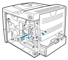
If you are replacing the network interface card with new one or the serial interface card, remove the two screws and the old card.
